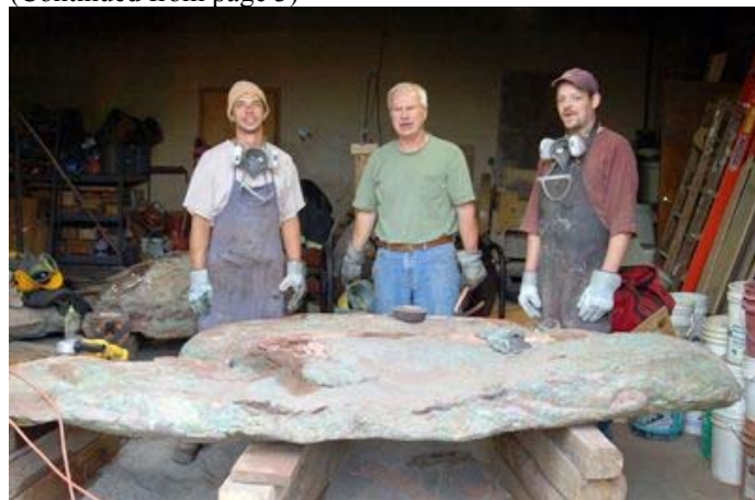
Figure 7. Chad Just, Ken Flood, and Jeremy Kerttu are “windowing” the chunk which entails grinding down the high spots and then sanding and polishing to highlight the native copper surfaces. Tom Rosemeyer photo (3 August 2017).
