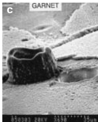
C was from a set of analyses of Fe-rich garnet from the Preissac-Lacorne batholith (this is the same garnet we used in the Hawley award Can. Min paper). 1064 nm. On this day, many of the pits exhibited an extraordinary build up of ablated material around the pit, forming a “sinter cone”-like structure. I have never seen this phenomenon again.
