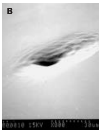
B was from the next set of ablations we ever tried – somewhat better ablation than A. Sample: glass slide.
